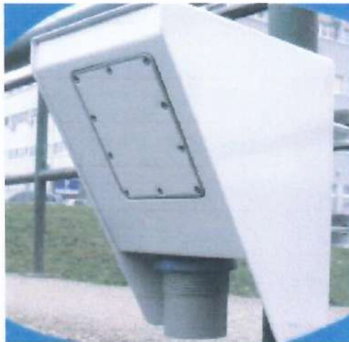
Figure 1: Example of Non-contact Open Channel Flow Velocity and Level Meter installed on a bridge
